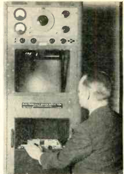
Shadow patterns of phase fronts near tiny models of antenna structures are shown on ground glass screen of this ripple tank
