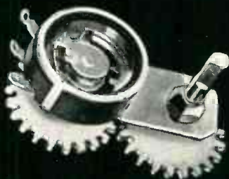
8 Control with offset shaft and operating gears.
