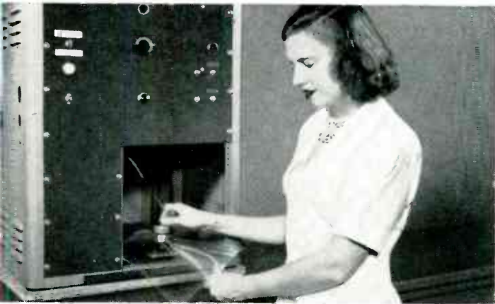
A voltage breakdown test of Kodapak Sheet.
