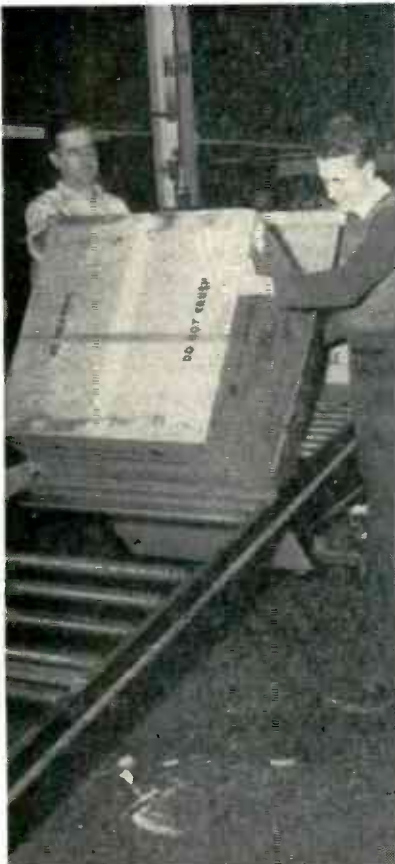
FIG. 3—Strategic omission of rollers and use of angle-iron stops in roller conveyor speeds and simplifies turning over of table-model tv sets in cartons for sealing of flaps
