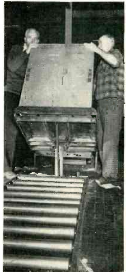
FIG. 2—Tilt table in roller conveyor line enables two men or even one to turn carton with 320-lb console on side for sealing of flaps. Here carton is being turned upright again after sealing
