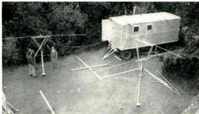
Receiving station for continuous-wave meteor clocking setup developed at Stanford University. Receiver overloading is prevented by a ground-wave cancellation system
