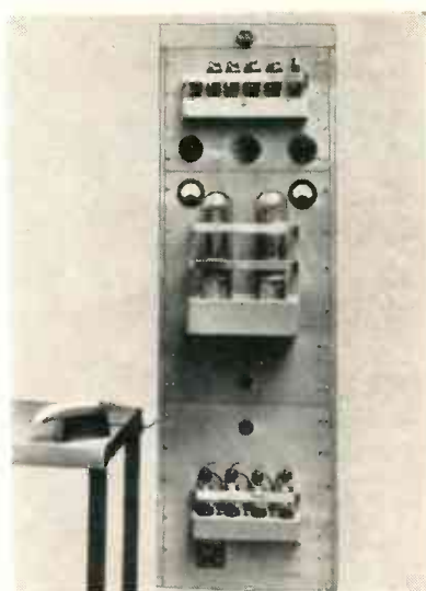
Driver stages and power supply of the generator. The tray mounted on the transducer is used for emulsification
