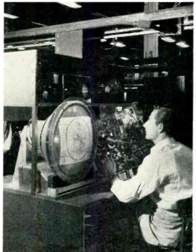
FIG. 16—Top of bench can be either sheet metal or plywood. The combination Lucite-metal holding fixture takes both 15-inch and 19-inch tubes
